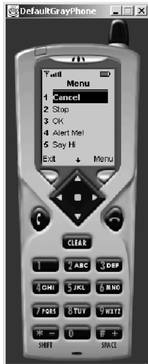
Figure 4.10. The MIDP implementation determines the policy for placing commands according to their type.
