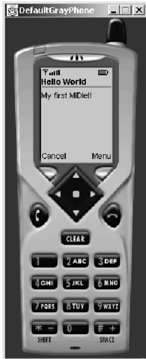
Figure 4.7. The implementation adds the "Menu" soft button when it detects more than two commands added to the current Displayable.
