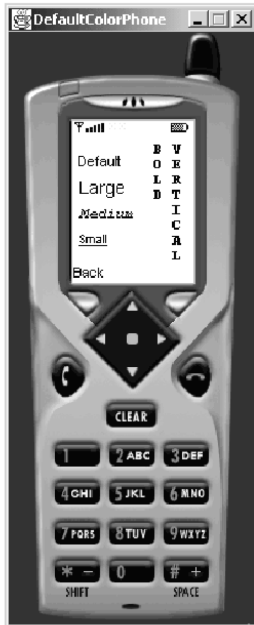
Listing 6.6 To draw text, specify the anchor point and the weighting of the anchor point. You can also specify the font of the text to be drawn.
