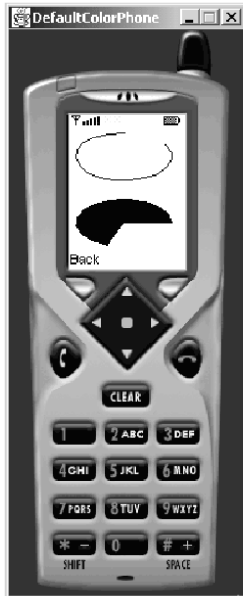
Listing 6.5 Arcs can be drawn in outline or in filled form, like rectangles.
