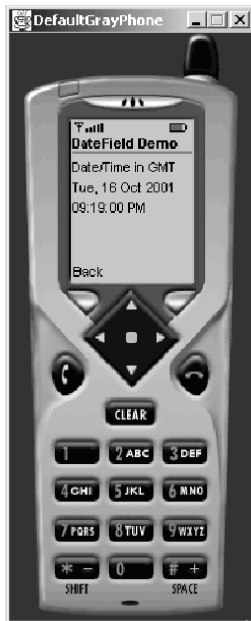
Figure 5.4. A DateField object consists of two parts: a label and a value that displays the quantity as text.
