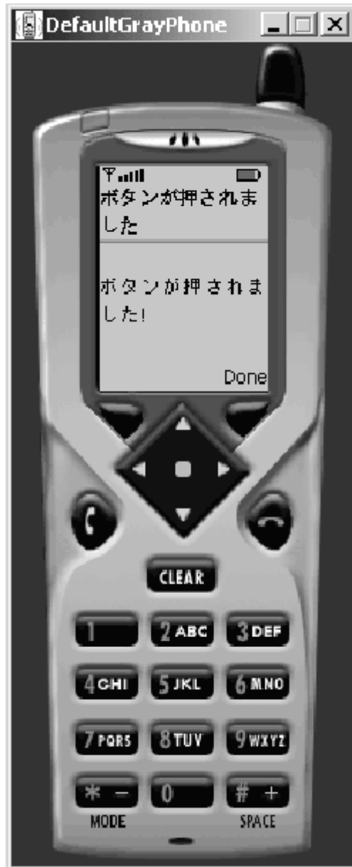
Listing 9.13 Unicode escape sequences accommodate all elements of all the world's written languages, including East Asian languages such as Japanese.
